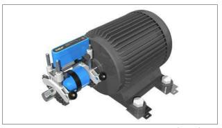
Mount the Measuring unit on the Moveable machine (Motor) side.
