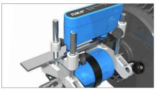
Adjust the gap between the inductive proximity sensors and the reference bar to app. 3 mm  $\pm 0.5$  mm (120 mils  $\pm 20$  mils). "Sensor status" in the app indicates the correct distance.
