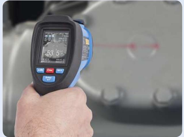
When used in non-contact mode, the thermometer senses the thermal energy radiated from an object with an infrared detector. When pointed at an object, the infrared detector collects energy, producing a signal that the microprocessor translates as a reading on the backlit display.
